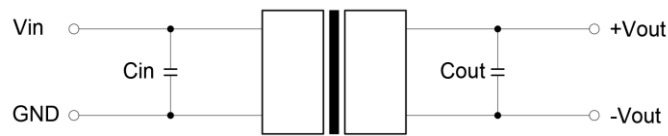
Figure 1: Typical External circuit
